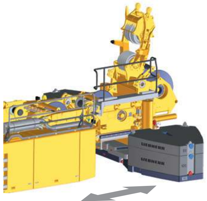
Luffing jib mode, counterweight radius 5.6 m or 6.6 m
